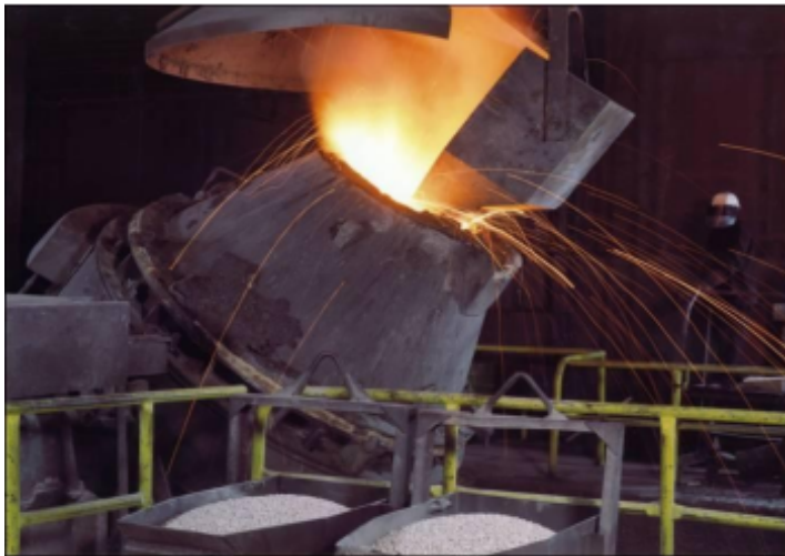
Ladle refining during conventional steel making process
