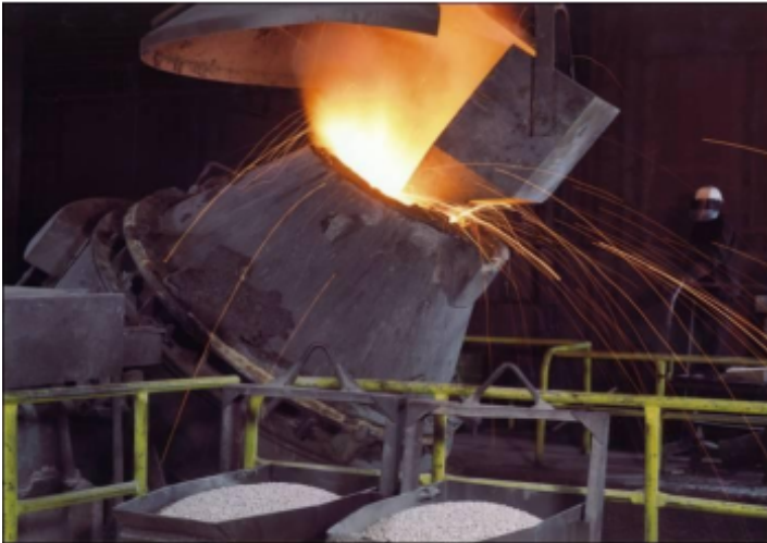
Ladle refining during conventional steel making process
