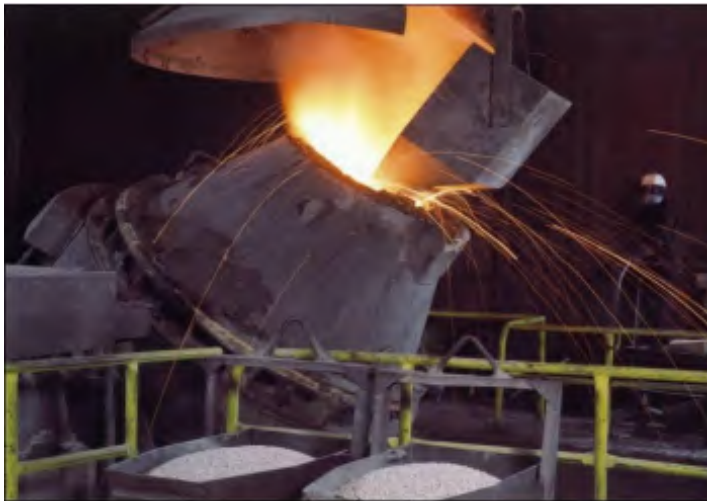
Ladle refining during conventional steel making process
