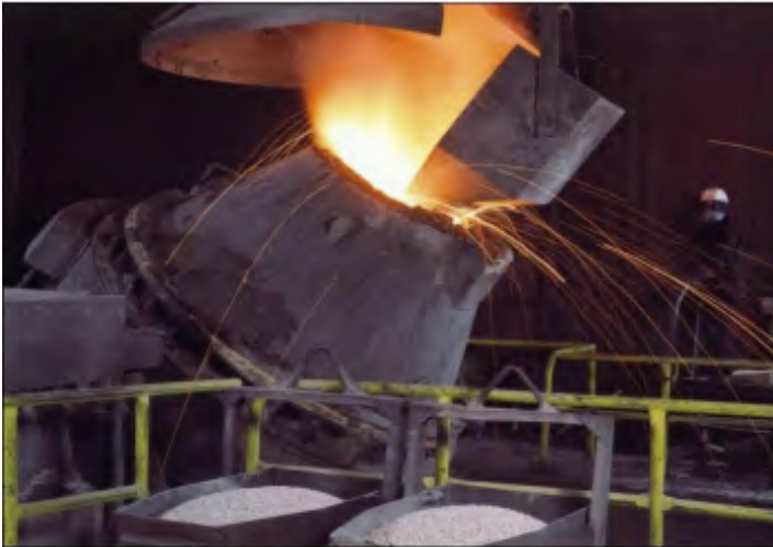
Ladle refining during conventional steel making process
